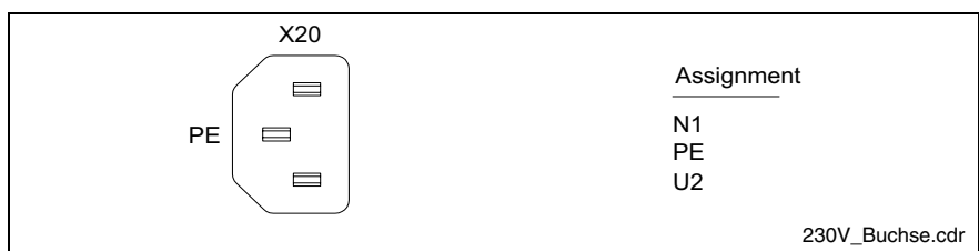
Fig. 7-18: Pin assignment of the 230/115 VAC connection X20
